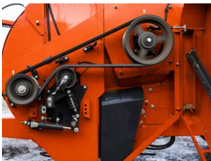
Flywheel can be run at full speed before the shredder drums are activated and material is being fed into the flywheel housing.
