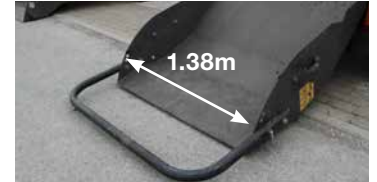
Wide tailgate design offers easier loading of bales.
