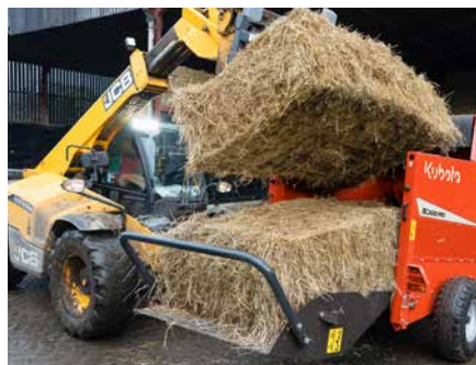
BC2600 PRO, offers an open-design bale chamber for easy access when loading from the top.
