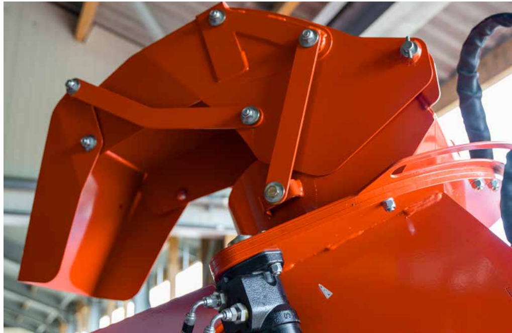
The swivel chute offers a 260° rotation of the chute.
