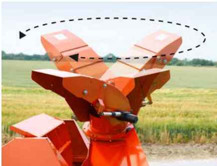
The swivel chute offers a 260° rotation of the chute.
