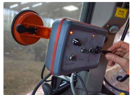
The 4-stage swivel chute is operated by the intuitive controlbox joystick.
